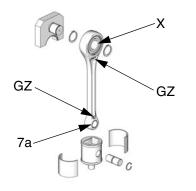
FIG. 9. Lubricate Wrist Pin Bearing Every 6 Months
